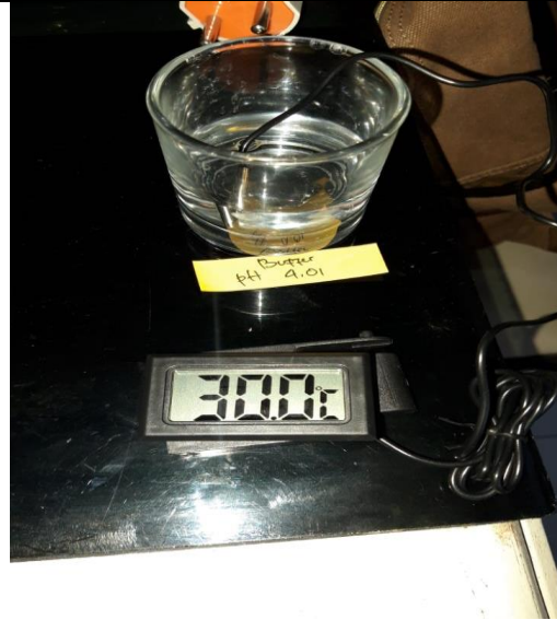
Proses Kalibrasi Sensor
