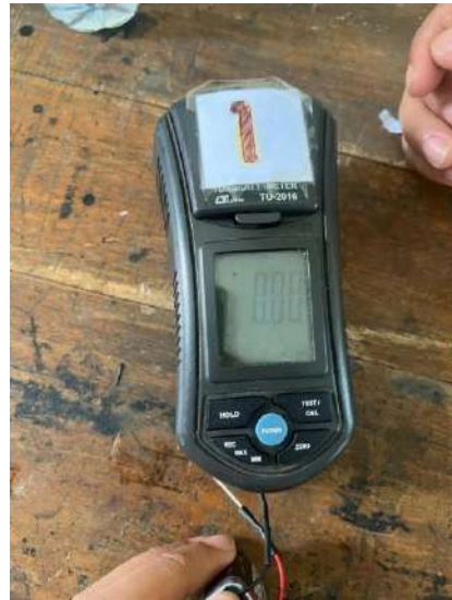
Pengecekan kualitas air kolam renang Turbidity
