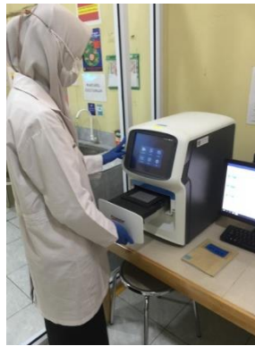
Masukkan tube kedalam mesin Real-Time PCR
