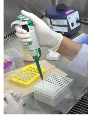
Masukkan 50 \mu l DNA kedalam tube Real-Time PCR
