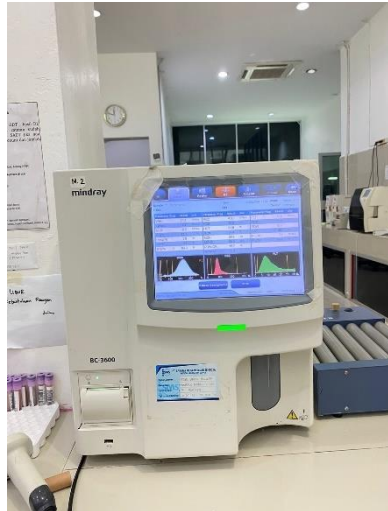
Gambar alat Hematology Analyzer BC-3600
