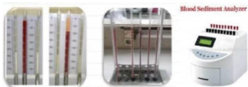
Gambar 2.5 (a). Metode Wintrobe (b). Metode Westergreen (c). LED Analyzer
