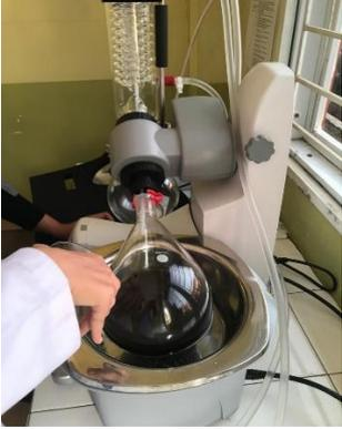
A rotary evaporator is shown in a laboratory. A glass flask containing a dark liquid is being rotated by the machine. A person's hand is visible, adjusting the flask. The machine has a white base and a glass condenser. The background shows a laboratory window and some equipment.               |
