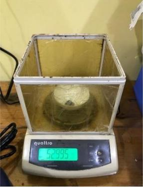
A digital analytical scale with a glass enclosure, showing a reading of 5.2995 on the display. The scale is white and black, with a green LCD screen. The brand name 'quattro' is visible on the front panel. The scale is placed on a wooden surface. |
