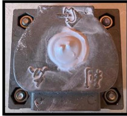
Gambar 3.11 *Flasking Cuvet Atas*
