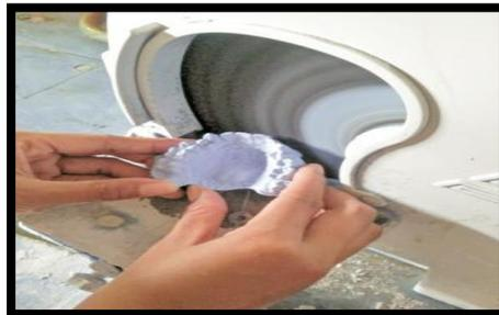
**Gambar 3.3** *Trimming Model.*
