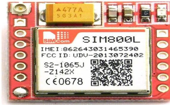
Gambar GSM SIM800L
