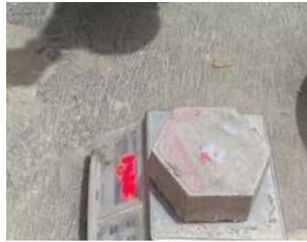
Proses Penimbangan Paving Block
