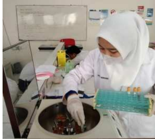
Sampel dicentrifuge 3000 rpm selama 15 menit
