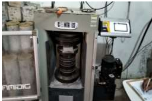
Proses Uji Kuat Tekan Paving Block Kontrol
