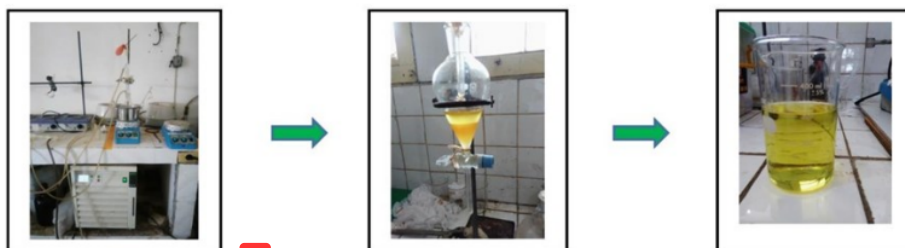
Figure 2. Preparation scheme of biodiesel made from waste cooking oil using CaO heterogeneous catalyst.
