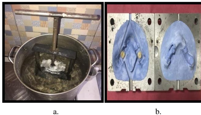
Gambar 3.13 (a) Proses *boiling out* (b) Hasil *boiling out*
