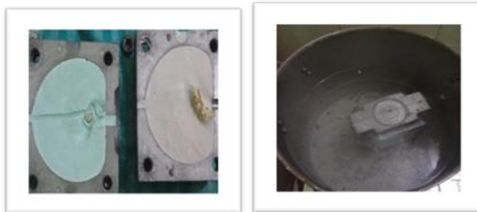
Gambar 3.12 a) Hasil Boiling Out (b) proses Boiling Out
