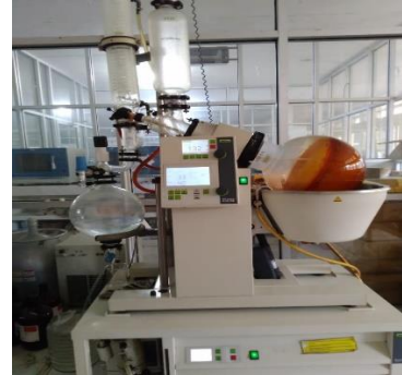
Evaporasi (Rotary Evaporator)
